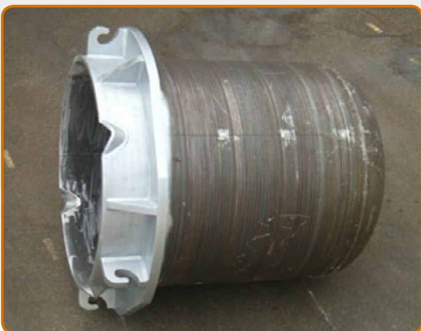
4. Crucible for recycling of magnesium alloys.
