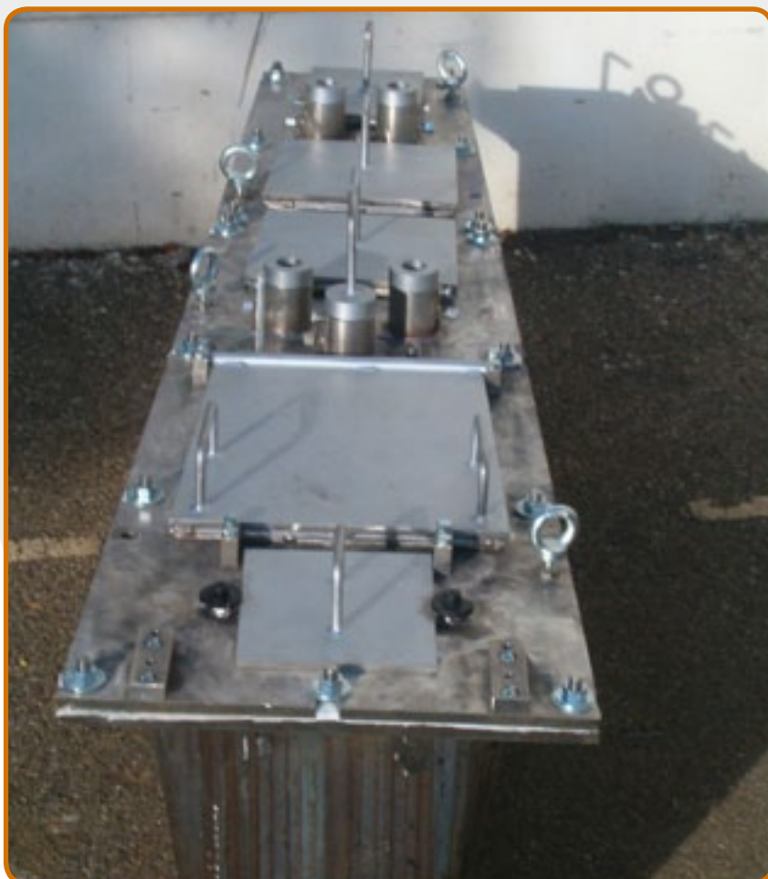
8. Crucibles for magnesium alloys for cold chamber die.
