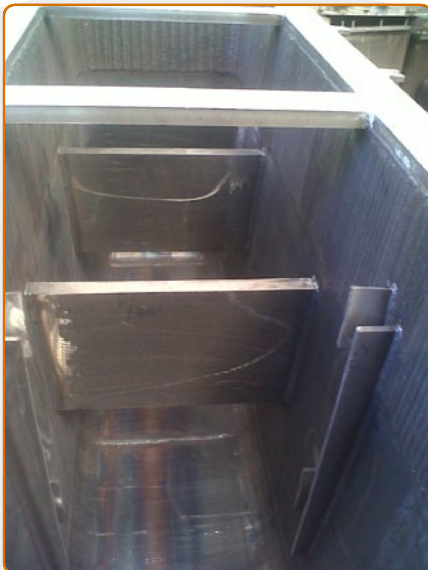
9. crucibles for recycling of magnesium alloys, 2.2 ton capacity.
