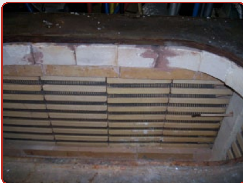
14. Electric heaters spiral of strip.
