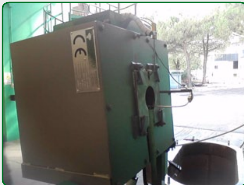
2. Furnace for reversible mg alloys for research laboratories.
