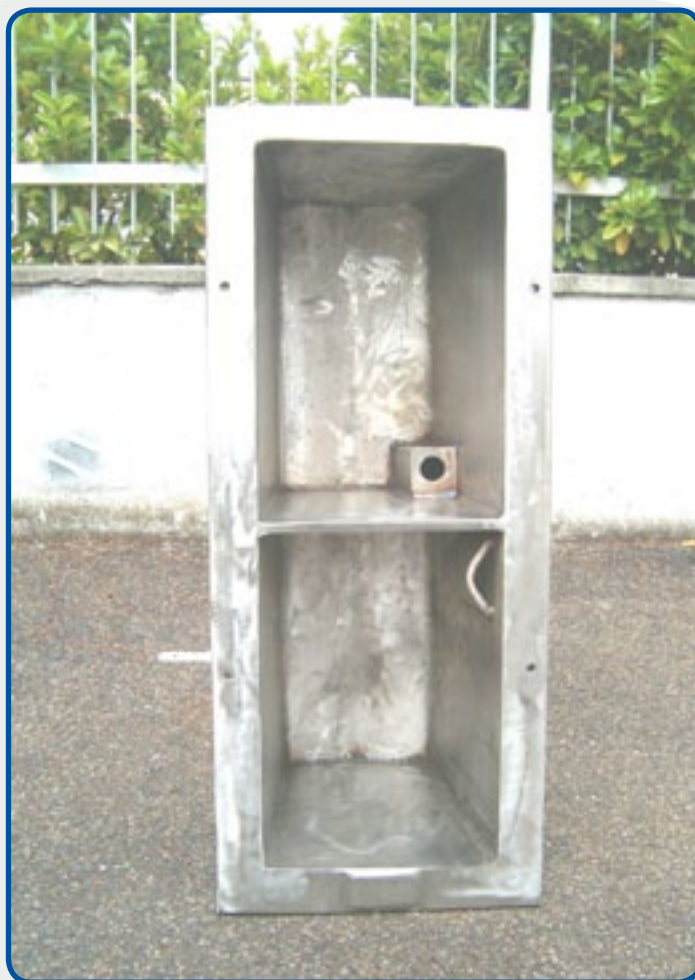
7. Double chamber crucible for zink alloys diecasting.
