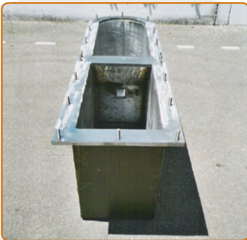
7. Crucibles for magnesium alloys for die casting hot chamber .
