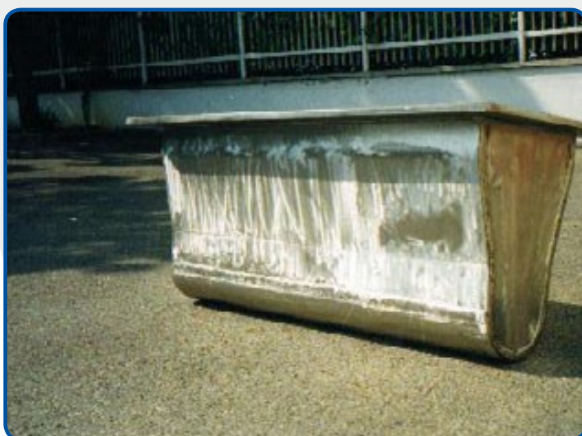
16. Remelting crucible for zink alloys, capacity 2500 kg.
