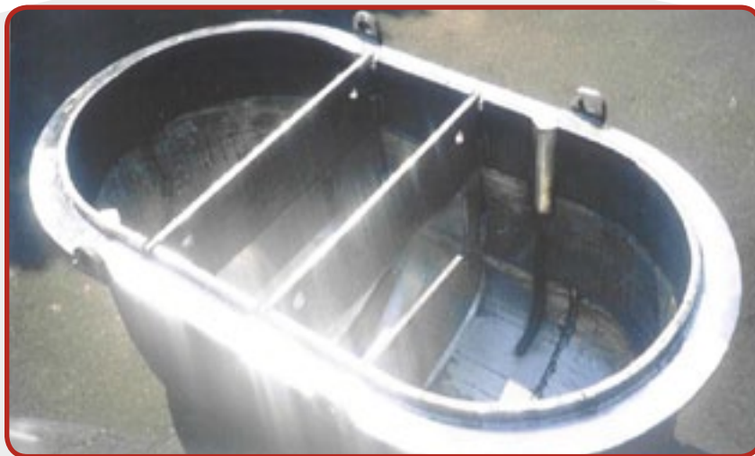
17. Double and removable parting wall, and a pocket for crucible thermocouple for die casting (dimensions and details according to customer's request).
