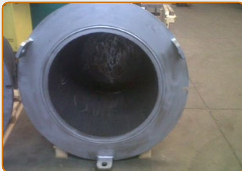
13. Crucible for melting in gravity, capacity 500 kg.
