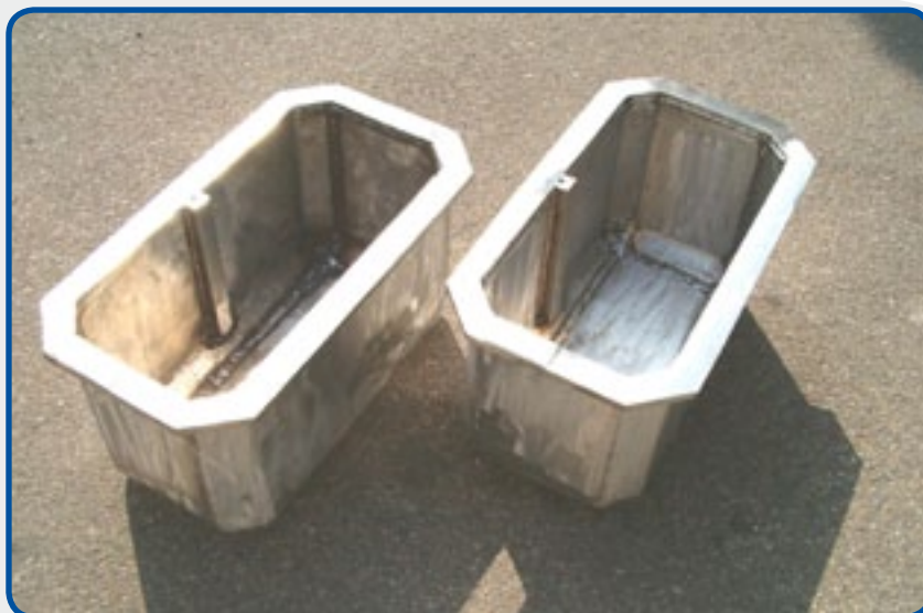
11. Crucibles for casting of zink alloys.
