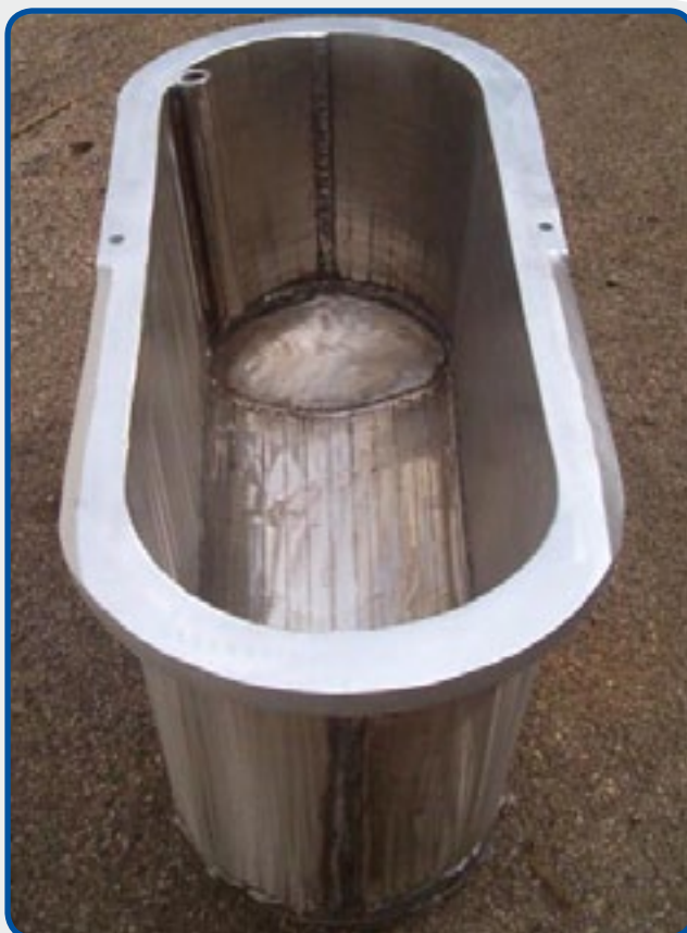
15. Crucible for casting of zink alloys, capacity 380 kg.
