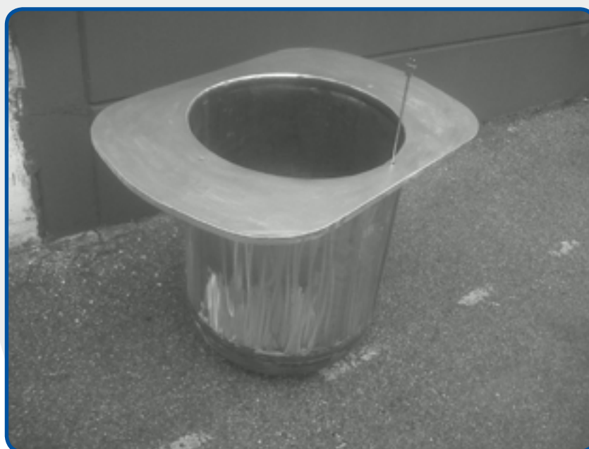
2. Crucible for special applications: pure zink.
