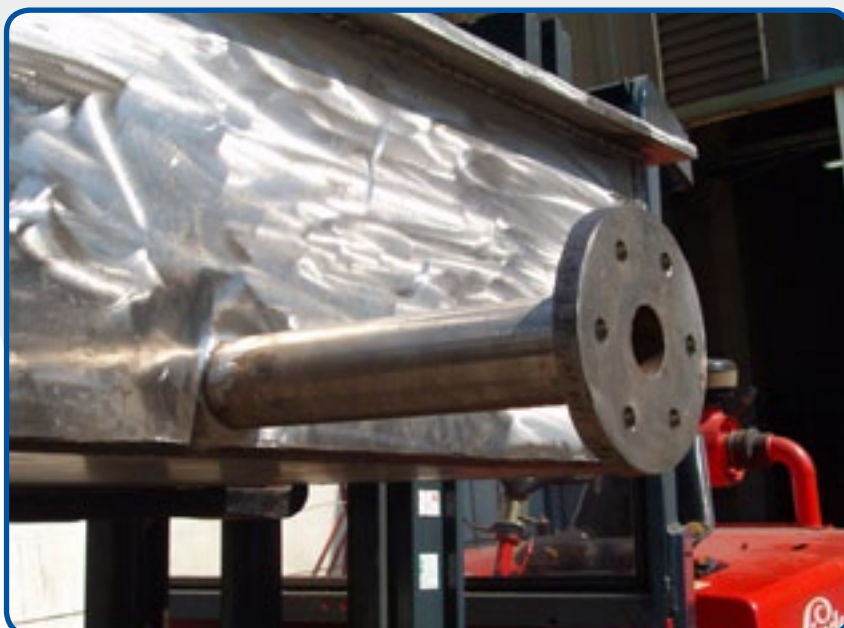
8. Crucible, capacity 10 ton of zink alloys with special valve.
