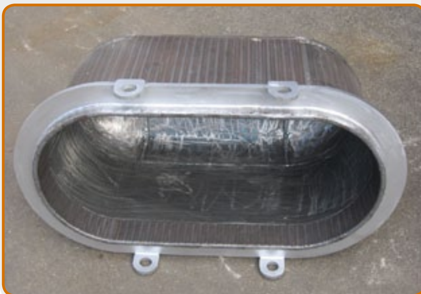
24. Crucible for magnesium alloys, 4 ton capacity.
