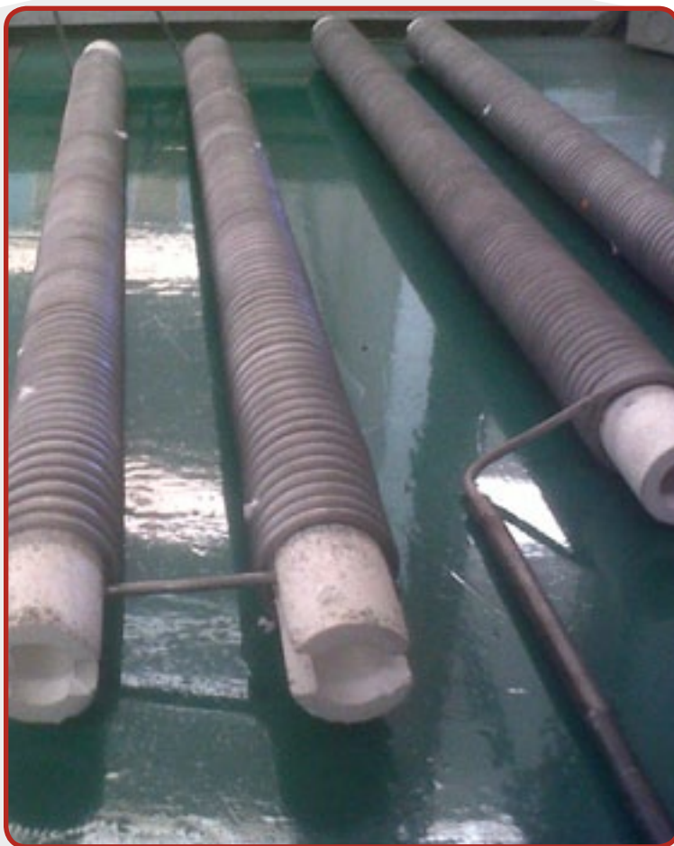
13. Electrical heating elements wound on ceramic support.
