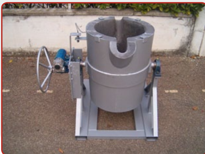
8. Transfer motorized ladle for Al (dimensions and details according to customer's request).
