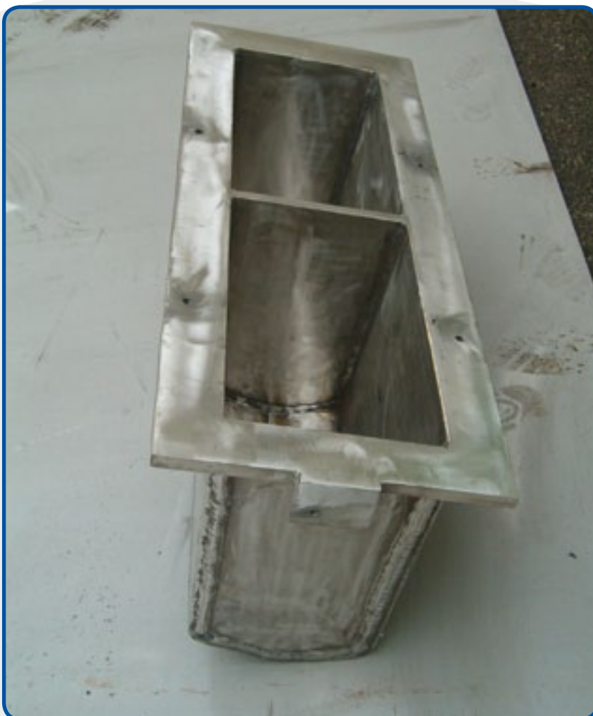
5. Double chamber crucible for diecasting of zinc alloys.
