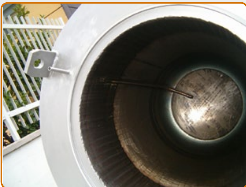
20. Crucible for magnesium low pressure casting.
