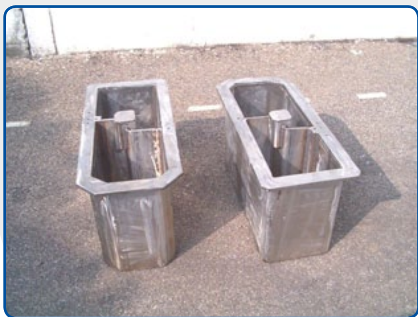
4. Double chamber crucible for diecasting of zink alloys.
